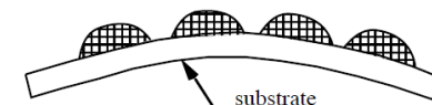
Attachment to the substrate restrains lattice expansion and this leads to compressive stresses in the film.
